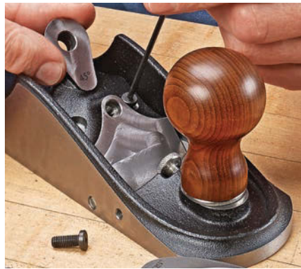
▲ The frog is held in place with a pair of cap screws. The toe plate is used to align the frog during installation.
