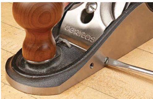
▲ A set screw on each side of the plane allows you to center the blade in the mouth opening. You typically only make this adjustment once.
