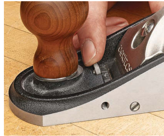
▲ An adjustment screw serves as a stop to prevent the toe plate from damaging the blade when adjusting the mouth opening.
