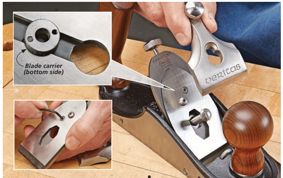
▲ The blade carrier nestles in the blade slot (top inset) and is secured to the blade with a single screw. The cap iron is attached to the blade carrier with a pan head screw. Adjusting the position of the carrier on the blade can be done with the cap iron installed (bottom inset).
