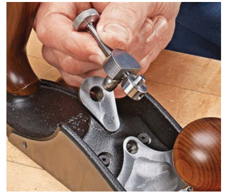
▲ The bottom pin on the adjuster mechanism snaps into the frog and is held secure by an internal retaining spring.
